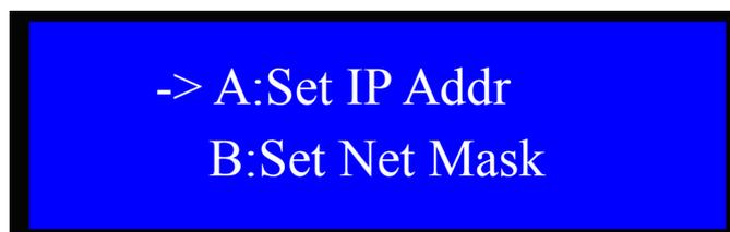
Press UP/DOWN to set different parameters for A/B/C/D/E, press key ENTER to return to previous menu, and key FUNC to enter the mode of setting different parameters.
